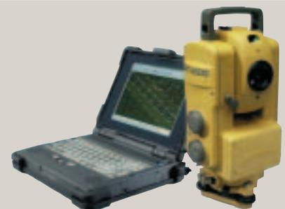
Auto tracking total station GRT-2000 for 3D machine control
